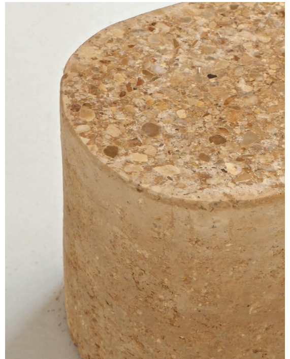
Compressed Earth Block, Syn Architects, 2023 Sample Courtesy of Earthman
